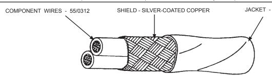
LOW OUTGASSING, RADIATION-CROSSLINKED, MODIFIED ETFE
